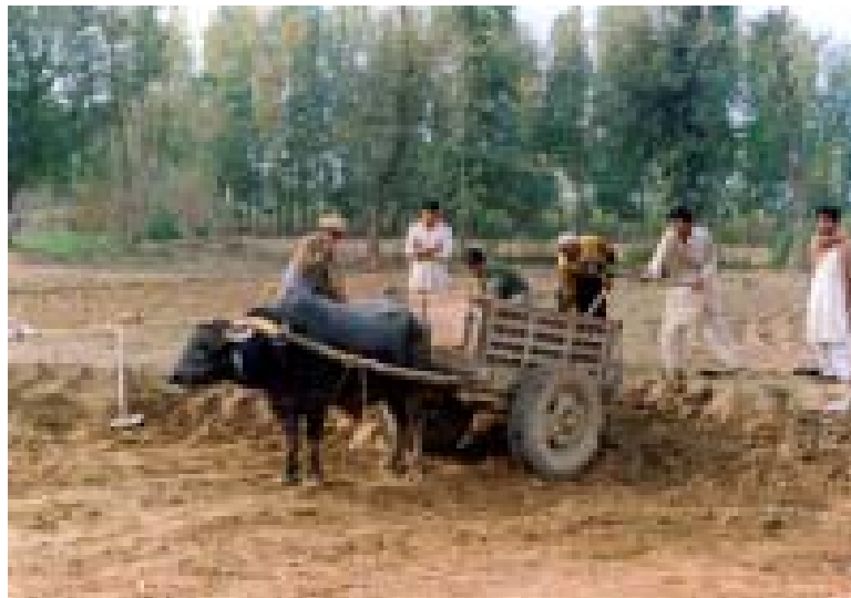
Figure 10. Cart with a special purpose body: earthmoving in Pakistan - the wide section pneumatic tyres are ideal for soft(ish) soil conditions.
