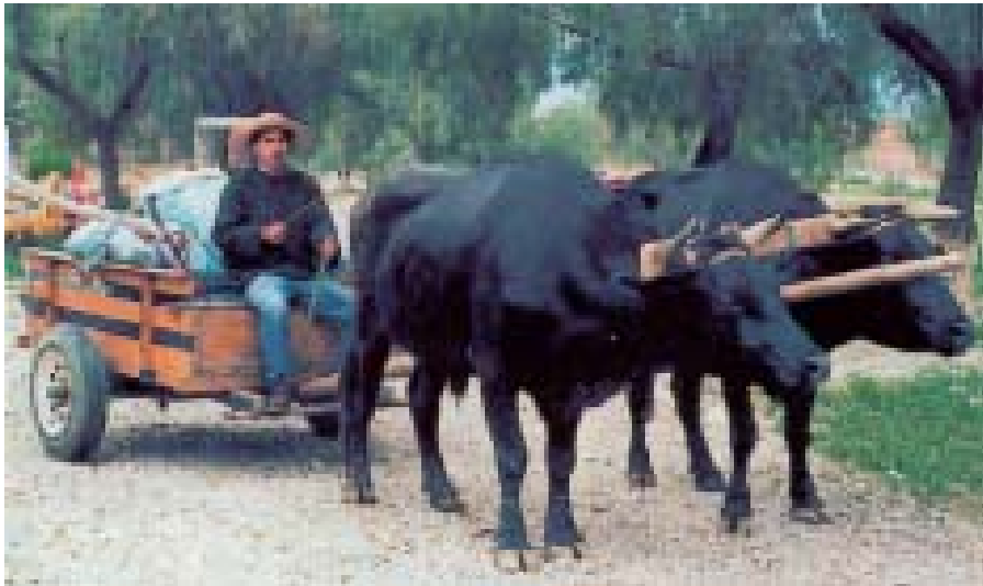
Figure 11. Single axle ox cart in Bolivia - fitted with external band brake on each wheel which can be operated when sitting at the front of the cart or when walking along at the rear.
